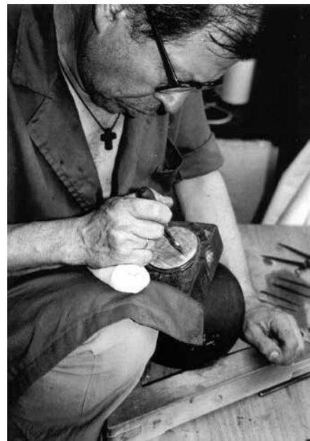
*Scoring the surface of a plate in preparation for later work.*
