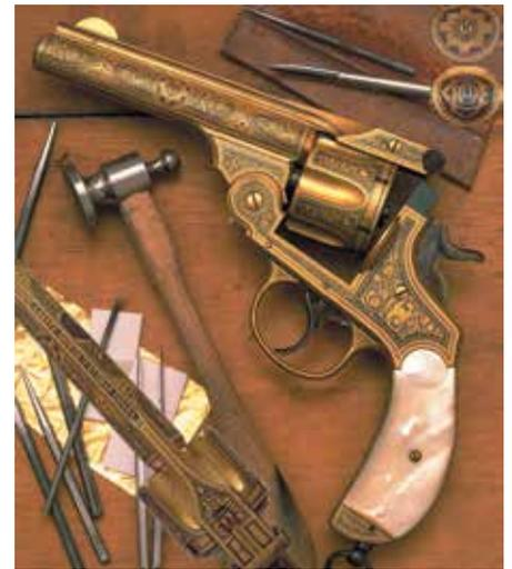
Garate, Anitua y Cia, sold a small number of .455 caliber revolvers to the British government during WWI. This example, an OP No. 1 Mark I prepared by F.A. Larrañaga, featured the "Order of the Thistle" on the left barrel, a symbol also used by the Scots Guards. Above the revolver is a burnishing tool. A selection of damascening punches and a mallet is grouped to the left.
