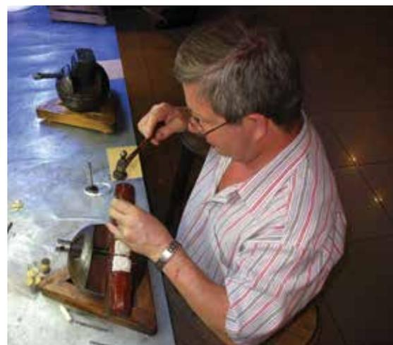
*Artisan working on pieces of jewelry. Work is fixed in resin, attached to a wood block, and positioned in a heavy ball vise.*
